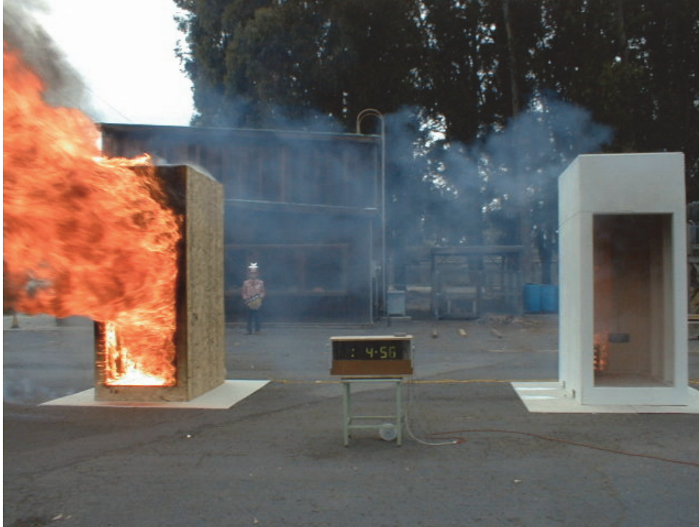
Figure 2-16 Intumescent paint test conducted by San Francisco Department of Building Inspection. Note large fire in unpainted building on left, little/no fire growth in intumescent painted building on right, both at 4:55 minutes following ignition.
