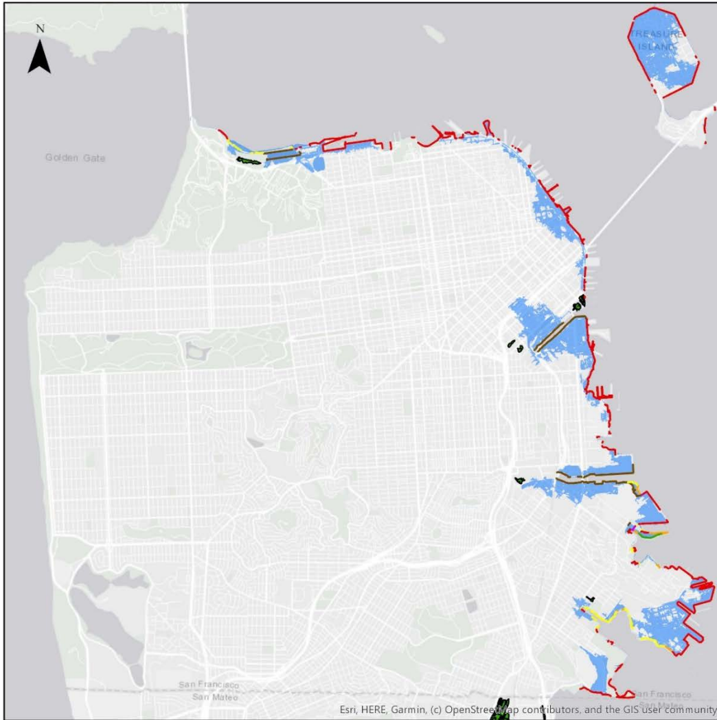
FIGURE A-64: SHORELINE PROTECTION AND FLOOD HAZARD (100 YEAR STORM + 24" SEA LEVEL RISE)
